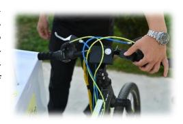
"Our device is composed out of 3 boxes, the central box where the battery is located, the box with the circuit board containing the switch, and a box with a joystick for giving commands that are displayed at the back of the bike." – continues Nikola Atanasovski.
